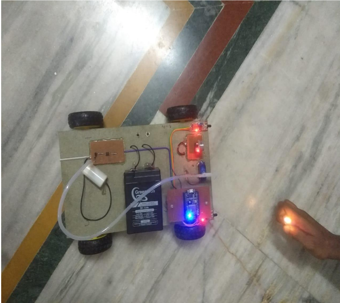
Fig 5.1 Robot when Detects fire
